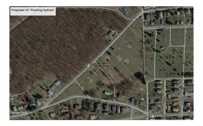
The 14" Flushing Hydrant project consists of tapping the main feed line from the Harding Street elevated tank. The tap and flushing hydrant will be placed at the low point on Walnut Street near the cemetery. This hydrant will allow the 14" line to be flushed to help improve water quality.
